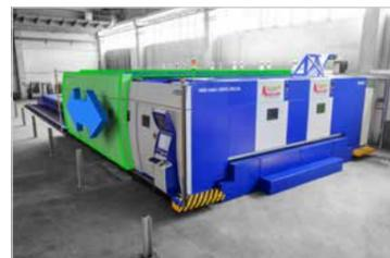
To accommodate its unconventional work areas while maintaining high safety standards, MSF Max uses a mobile safety cabin to shield against laser beam reflection. The mobile cabin moves on its own guidelines and can reach the entire work area of the machine. Optionally, a retractable version of the mobile cabin allows to choose different work area sizes and thus enables an unmatched flexibility of operation.
