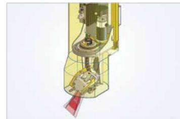
For cutting of hollow sections, the PipeCut machine can be equipped with a laser scanner that will measure the deviation of profile's position in the place of cutting to ensure precise positions of cut-outs and openings.
