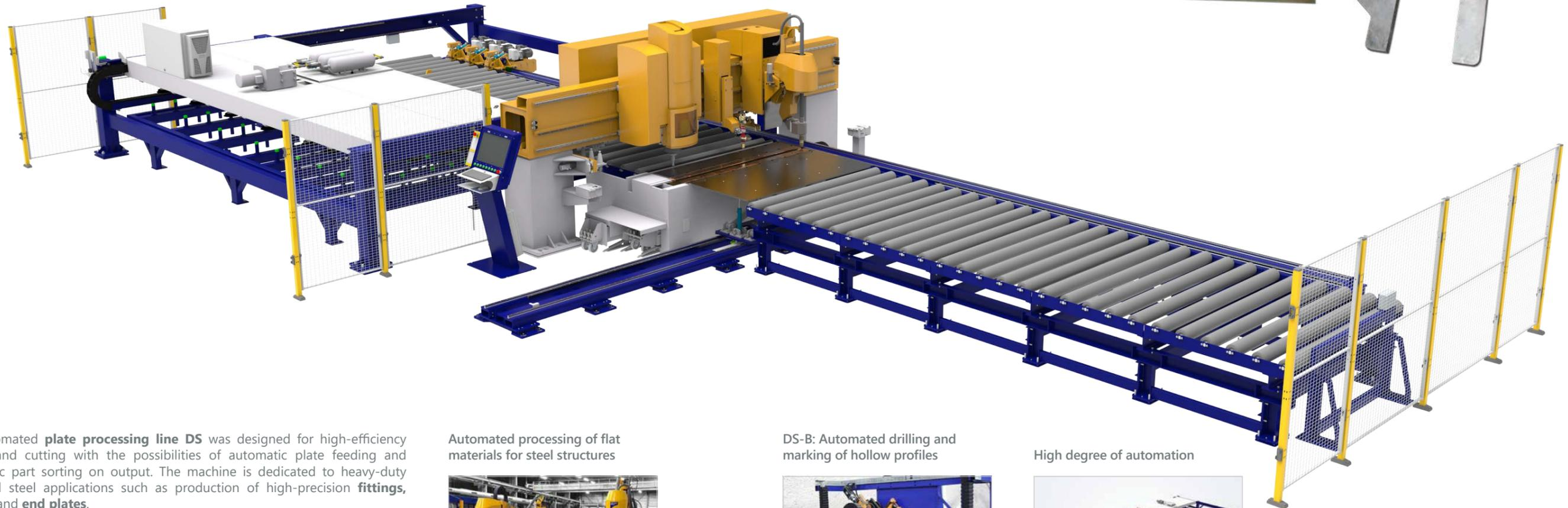
The automated **plate processing line DS** was designed for high-efficiency drilling and cutting with the possibilities of automatic plate feeding and automatic part sorting on output. The machine is dedicated to heavy-duty structural steel applications such as production of high-precision  **fittings, gussets and end plates.**
