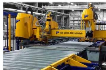
The DS series offers a variety of automated processing options for flat materials. Besides drilling, 2D and bevel cutting for weld edge preparation up to 50°, oxyfuel cutting, tapping, countersinking as well as scanning and marking are possible. The standard work area size is up to 6,000 x 2,000 mm.
