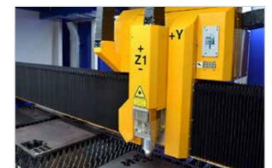
MicroStep relies exclusively on high-quality components from established manufacturers to ensure long-lasting and accurate results. Thus, laser sources from IPG Photonics with a power of up to 4 kW are available. For high cutting speeds, an automatic laser cutting head from the German manufacturer Thera-cut is used.
