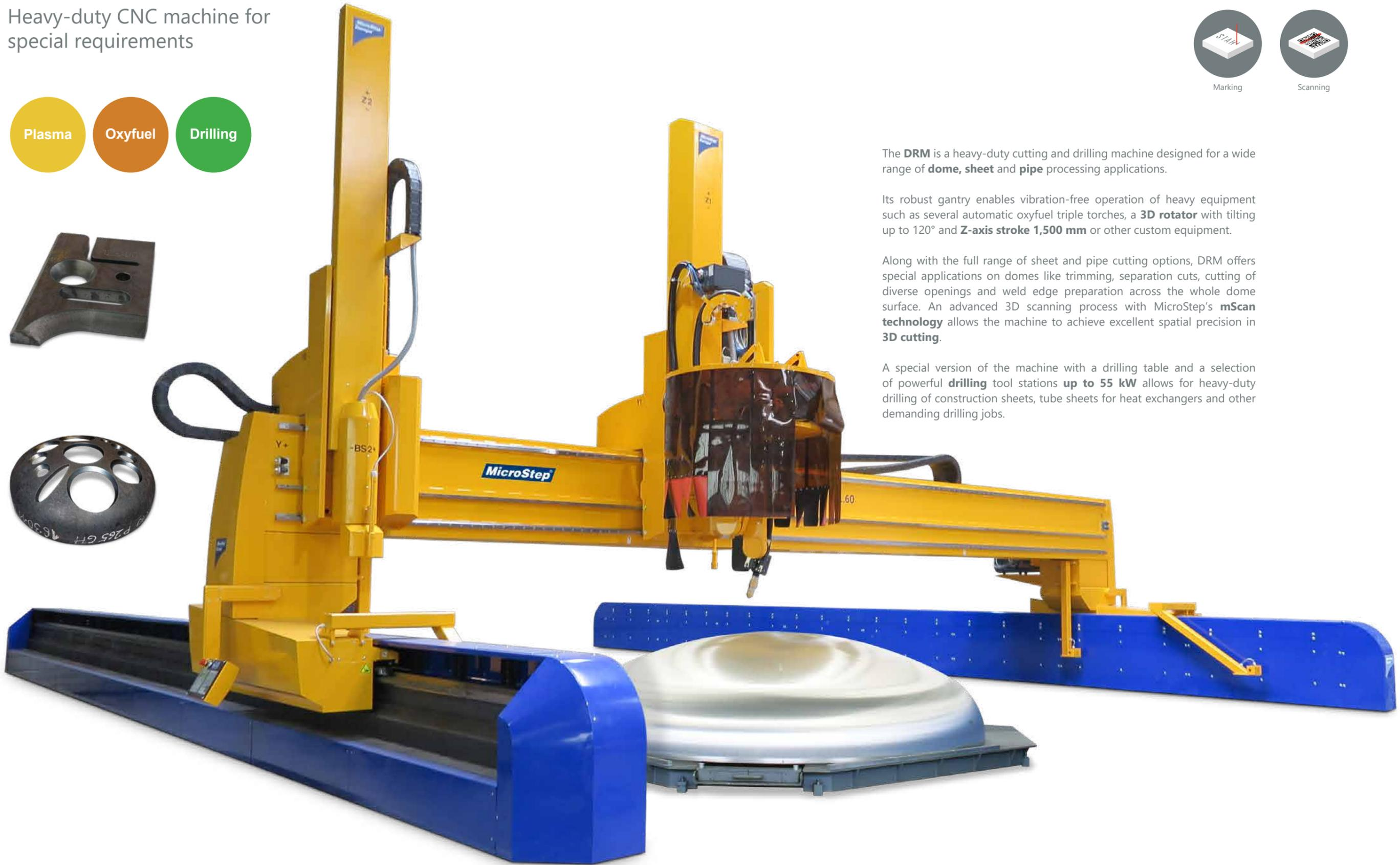
The **DRM** is a heavy-duty cutting and drilling machine designed for a wide range of **dome, sheet** and **pipe** processing applications.
