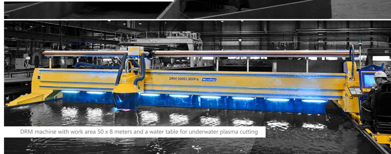
DRM machine with work area 50 x 8 meters and a water table for underwater plasma cutting
