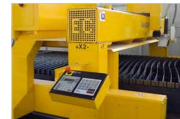
A standalone, ergonomic MMI console provides the operator with an overview of all cutting processes, machine related information as well as extensive multi-tasking features. Additionally, a handy operational panel on the gantry allows the operator to perform basic tasks such as interrupt a cutting program, initialize or move the machine or perform a manual cut.
