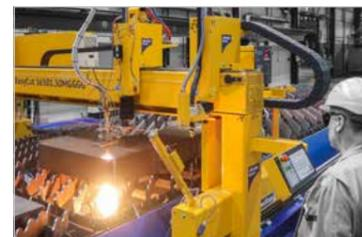
EasyCut machines are designed to withstand high workloads in multiple-shift operations including multi-torch parallel oxyfuel cutting of material thicknesses up to 300 mm. Intelligent temperature management keeps the system from exceeding its limits even in harsh environmental conditions and under intensive cutting load.
