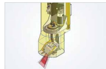
ProfileCut machines are equipped with a 3D laser scanner that measures the exact shape of beam in the place of cutting. Advanced algorithms then allow the control system to adjust the movement of tool accordingly and compensate for possible inaccuracies of the particular beam.
