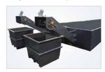
The cutting tank can be optionally equipped with an automatic cleaning system, either with a conveyor belt that carries the sludge to a sludge container at the end of the cutting table or with an automatic system for filtering out the abrasive.
