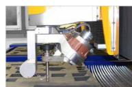
In order to meet the requirements for high precision and/or perpendicularity of the cut parts, MicroStep's Adaptive Bevel Compensation (ABC) technology enables taper compensation in a range of  $\pm$  7°. The technology adjusts the bevel angles with speed to compensate the natural stream lag and taper of a water jet. The system also allows custom adjustment of the compensation values.
